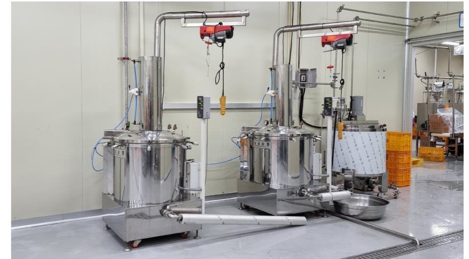
Juicer Crushed fruits are located into a sack and juiced by a juicer. Equipment Juicer.
