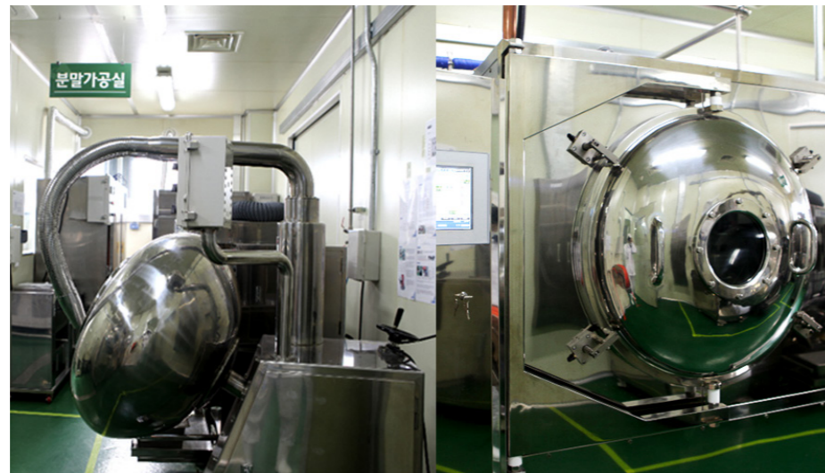
Powder Processor Dehydrating raw materials and crushing/blending, pellet making, powder processing, and other high tech raw material processing units are in possession. Equipment Low temperature lyophilizer, blender, mixer, pellet maker
