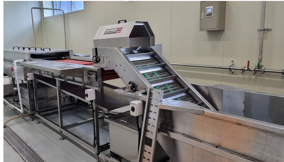
Fruit Washer Fruit washer for pears, apples, peaches, and other large sized fruits. The fruits are drenched in water and bubble washed for initial washing process. Then the fruits are moved through a conveyer and washed with thoroughly sprayed water, resulting in hygienic materials for production. Equipment Fruit washing machine.
